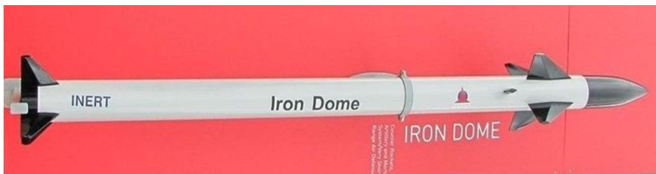
An example of an interceptor Tamir missile used in Iron Dome System.
